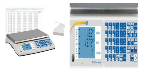
Professional counting scales up to 3 kg / resolution from 0.1 g / triple display / Memory for up to 1,000 articles / monitoring of the number and weight of pieces / Scanner, USB, PC, printer connection / optional OC switching contacts, 4-20 mA, 0-10 V
