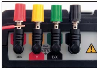
Terminal Adapters are used to allow the DET4 Series units' terminals to accept alternative cable connections.
