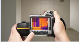
Infrared cameras quickly locate moisture related problems
