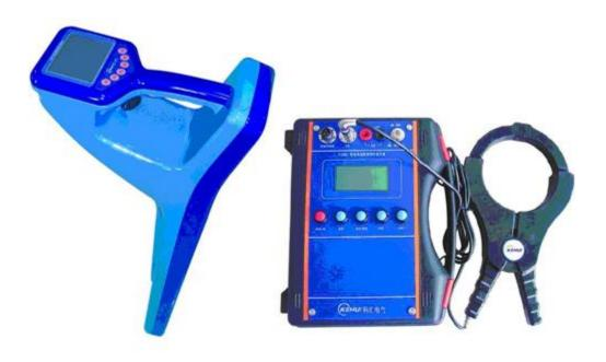
T-200 Cable and Pipe Locator consists of a transmitter and a receiver, it can be used to locate trace and depth of the underground cables and metallic pipes, it can also be used to identify the cable from a group of cables.
