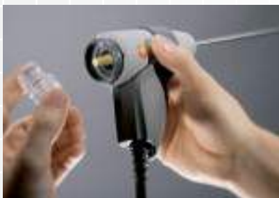
Easy-to-change particle filter built into probe handle
