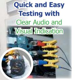
Based on the electrostatic induction theory, the 3129 series Phase Detectors can safely and accurately detect phase rotation in three-phase circuits. Correct rotation is indicated by a crystal clear beeping tune, while bright red LEDs show rotation direction.
