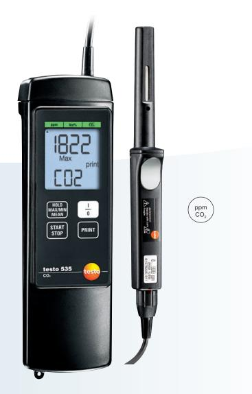
Bad air quality in indoor rooms due to excessively high  $CO_2$  concentrations (greater than 1000 ppm) leads to tiredness, lack of concentration and can even cause illness. testo 535 is a precise, reliable  $CO_2$  measuring instrument for monitoring Indoor Air Quality. The high-quality and stable 2-channel infrared sensor allows long-term measurements, and does not require repeated adjustment.
