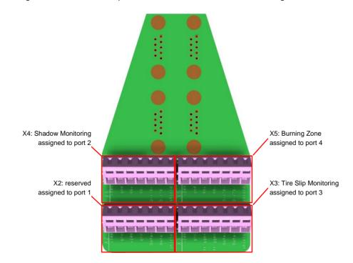
Note It is not recommended to change the pre-set configuration for the four ports of the serial device <XXXSYSCS210CON>!
