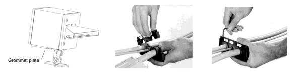
Using the 4 M5x25 screws, mount the grommet plate on the outside of the protective housing. Plug the cable connectors into the linescanner. Connect the socket and the plug for earth ground.
