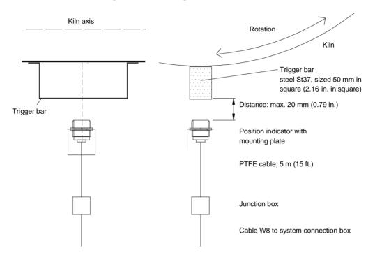
Figure 4-7: Mounting the Position Indicator
