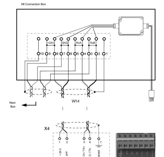
Figure 8-12: Shadow Monitoring – Wiring
