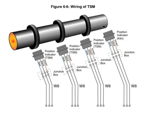
For the detailed wiring of the TSM see section 8.7 TSM – Wiring, page 54. For recommended cables see section 3.5 Cable Requirements, page 19.
