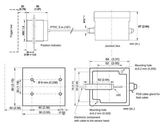
Figure 9-4: Dimensions of Position Indicator and Junction Box
