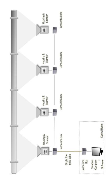
Figure 8-3: System Installation – Multiple Scanners
