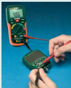
AC/DC Voltage measurements
