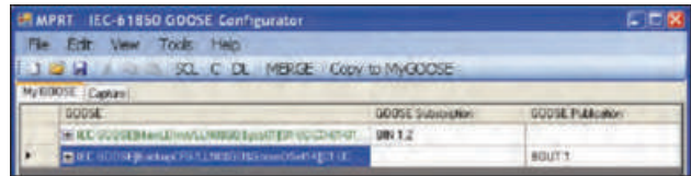
Figure 2 MGC 'My GOOSE' with Assigned Binary Inputs and Outputs
