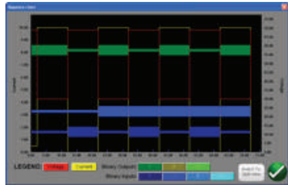
Sample Sequence Voltage, Current, Binary Inputs and Outputs
