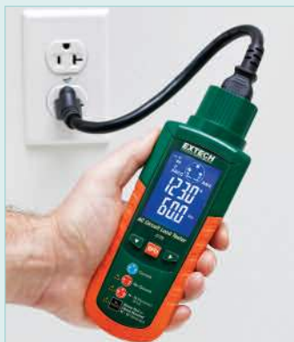
Tests 3-wire standard and GFCI receptacles
