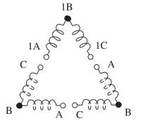
the group should be marked according to the MOTOR lead markers. The number 1 should be used as a prefix to identify the group. Thus, the terminal connected to the A MOTOR lead is marked 1A. The common terminal is marked 1B, and the remaining terminal is 1C.
