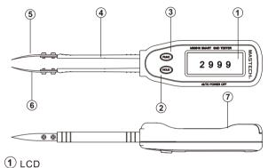
(4) Pin Holder (5) Test Pin(Gold-plated)('INPUT' Terminal) (6) Test Pin(Gold-Plated)('COM' Terminal) (7) Battery cover
