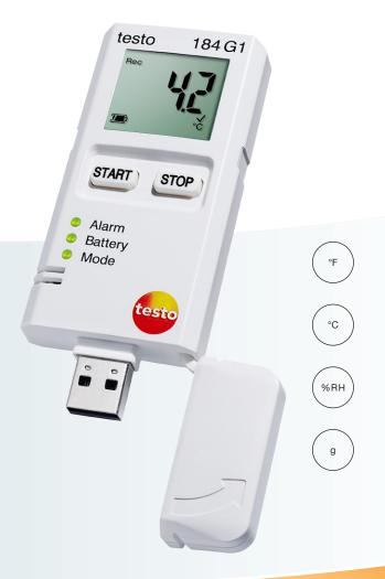
The data logger testo 184 G1 is designed specifically for the monitoring of shock, relative humidity and temperature during transportation. In addition to the precise temperature and humidity measurement, a 3-axle acceleration sensor measures any vibrations which occur.
