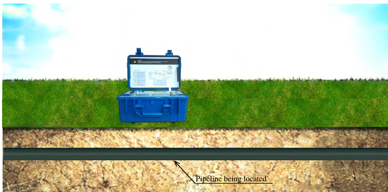
Figure 5 – Cable/pipeline location using closed-loop method
