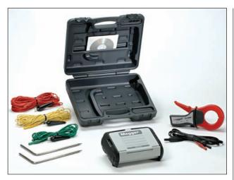
Each instrument comes complete with three sets of leads, two test spikes, instruction manual CD, and a rugged carrying case, (current measuring clamp, shown, is an optional accessory for performing the ART testing capability using the DET4TC2 and DET4TCR2 only.)
