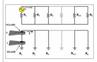
there is insufficient space to perform a classic fall-ofpotential measurement. In addition the units can be used to measure ground leakage or phase current.
