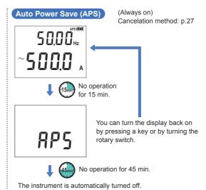
To restart the instrument, briefly set the rotary switch to "OFF."
