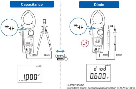
Intermittent sound: during forward connection (0.15 V to 1.8 V) backlight off
